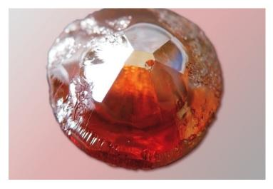
An aluminum nitride crystal which has to be produced as the basis for the UV LED.
