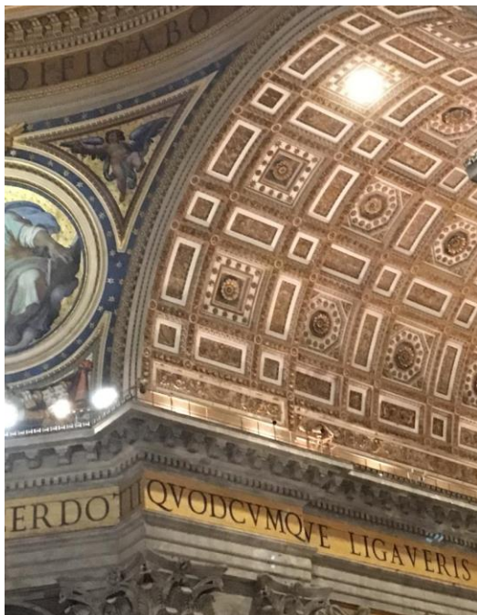
Left image, old illumination: The illumination throws a disturbing shadow on the inscription below.
