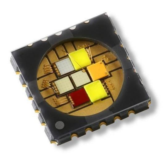
The LZ7 Plus from LED Engin, designed for stage fixtures, features seven high-power dies in six colors, which can be individually controlled to deliver intense, saturated colors, as well as high quality white light.
