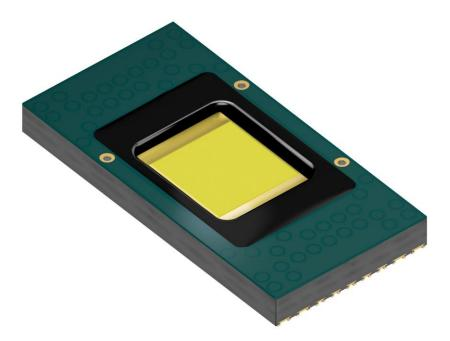
The Eviyos prototype is the first integrated hybrid LED in which a  $\mu$ -structured light emitting chip and individual pixel control have been combined in a single component. Picture: Osram
