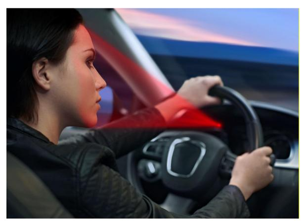
For driver monitoring the IREDs illuminate the driver precisely so that a camera can capture the drivers' status (drowsiness, distraction) and pass this information to the system.
