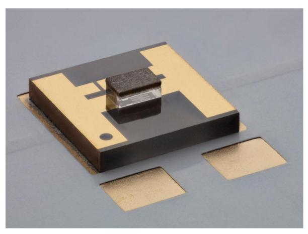
UV-LED in flip-chip geometry mounted on an AIN submount.
