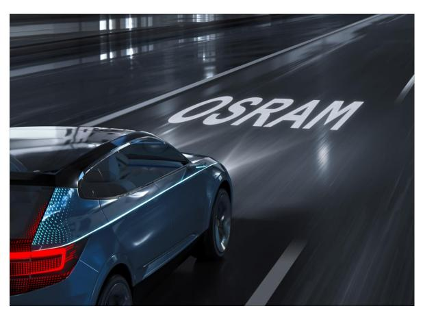
Visualization of information with the help of the headlight in HD quality - the 25,600 pixels of the second generation of Eviyos will make it possible in the future. Picture: Osram
