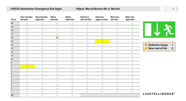
Thanks to OSRAM Lightelligence, testing of the signs can be carried out very simply – remotely with the press of a button. Supported by sensors, a software monitors the proper functioning of the safety signs from any location. Defective luminaires are registered by the software, as is the remaining lifespan of the operative lamps. This allows predictive maintenance, saving both time and money.
