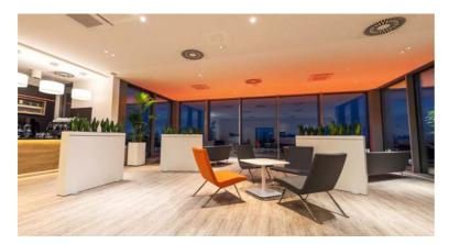
A relaxed atmosphere in the Skygarden is created by Lunis downlights and wallwashers with a warm light colour, light coves with flexible LED strips along the walls and Traxon Allegro RGB LED linear luminaires that illuminate the ceiling and the view from below with orange.
